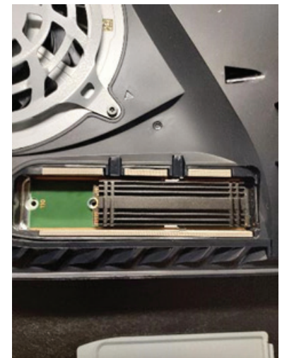
Crucial P5 Plus with M.2 2280 Heatsink inside Playstation 5 SSD Slot
